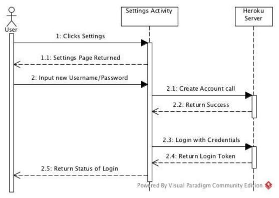
This diagram describes the steps taken by a user to create a new account. After settings is chosen, the settings activity returns the Settings page for the user to input new credentials. The settings activity then sends the credentials to the Heroku server. The server checks to make sure the credentials are valid, then returns a success. The activity continues to login in with the new credentials.
